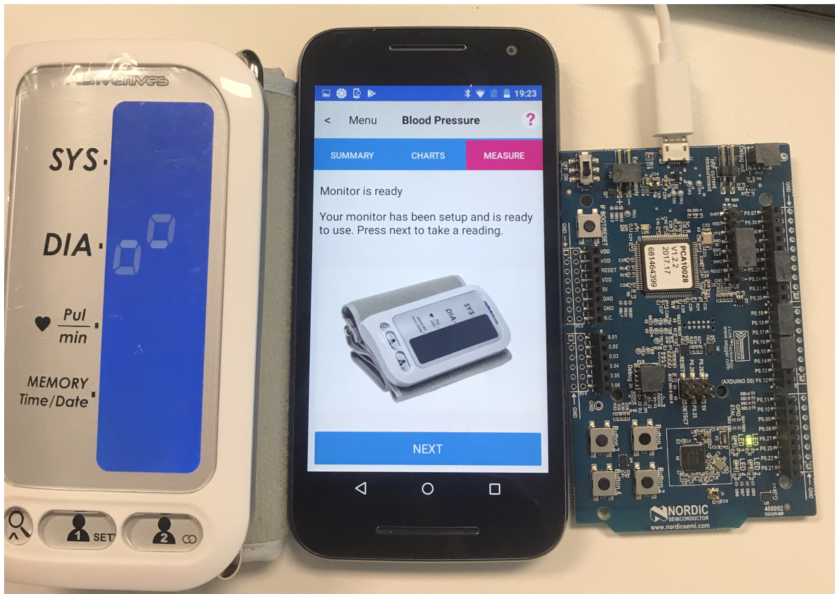
Figure 4.7: The application pairs with the fake BLE device (on the right) instead of the Blood Pressure Monitor.
