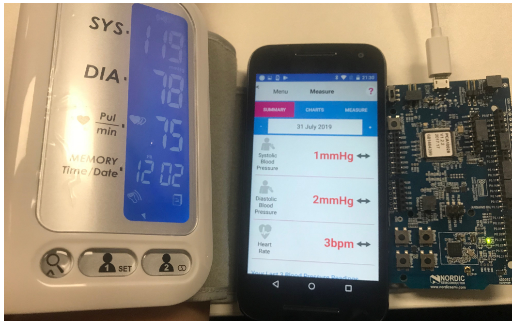
Figure 4.8: The application have received spoofed data from the fake BLE device instead of the actual reading measured with the blood pressure monitoring device.
